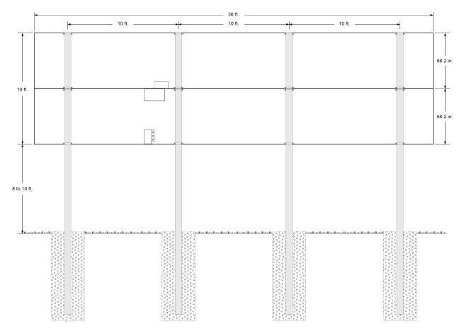
Once you have verified the positions of the posts and the size of the footings, you are ready to dig your holes, pour your concrete, and set your posts. There are several techniques for ensuring proper alignment of the posts. Typically installers will construct a temporary wooden support frame to hold each post in place while the concrete sets. Having plumb posts in the proper position is the key to a smooth mechanical installation.
